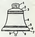
bell 1: crown, 2: head, 3: shoulder, 4: waist, 5: band lines, 6: sound bow, 7: lip, 8: mouth, 9: clapper
